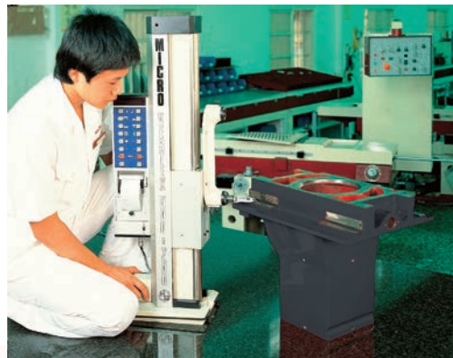
The parallelism of the wheelhead guideways is inspected with a precision electro-indicator.
