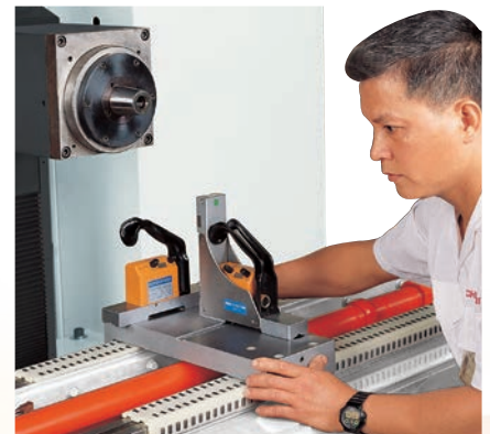
Parallelism and flatness of the table guideways are checked by "In Process Quality Control". These and numerous other tests throughout production help to maintain and improve the quality of Chevalier grinders.
