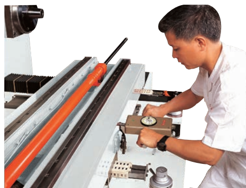
Driving force test on saddle
