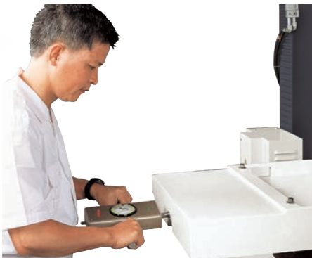
Driving force test on table
