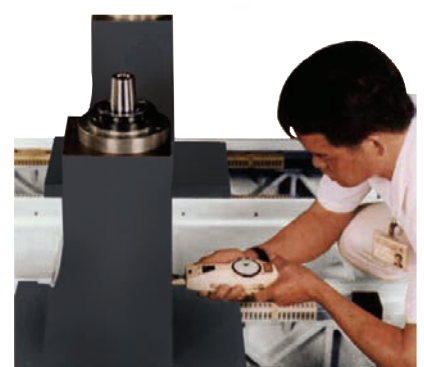
Driving force test on column
