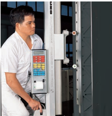
The column is placed on a granite surface plate and the perpendicularity of the guideways is inspected with a precision electro-indicator.
